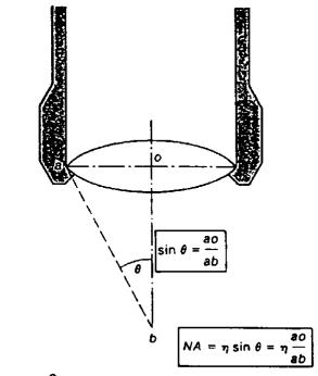
Figure 2 A diagrammatic representation of numerical aperture, (NA).
