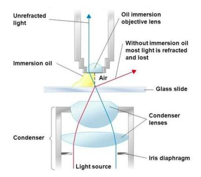
Figure 3. Comparison between the effects of immersion oil and air on the passage of light rays from a specimen to the front lens of the oil immersion objective.
